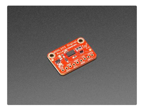
The ADXL343 is nearly identical in specifications to the ADXL345, and code written for the '345 will likely work on the '343 as-is. This new accelerometer has some nice price improvements to stay within your budget.
