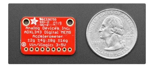
We added an on-board 3.3V regulator and logic-level shifting circuitry, making it a perfect choice for interfacing with any 3V or 5V microcontroller or computer such as Arduino or Raspberry Pi. We even have library and example code for both Arduino/C+ + and CircuitPython, so you can get started super fast with any platform!
