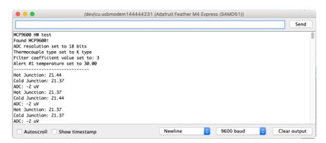
Note: The image above shows 9600 baud in the serial monitor. It should be 115200 to match the code!
