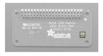
The default I2C address for the Bonnet is  $0 \times 74$ . Solder this jumper closed to change it to  $0 \times 70$  to avoid I2C address conflicts, if needed.
