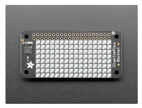
The IS31FL3731 is a nice little chip - and it runs happily over 3.3V power. Inside is enough RAM for 8 separate frames of display memory so you can set up multiple frames of an animation and flip them to be displayed with a single command. Since it uses I2C, it takes up only the SDA/SCL pins on your Pi and can share those pins with other I2C devices and sensors.
