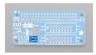
The MCP23017 has interrupt capabilities. There are two IRQ pins (INTA and INTB) you can solder a wire to, if you want to have a quick way of telling if any of the GPIO's changed.
