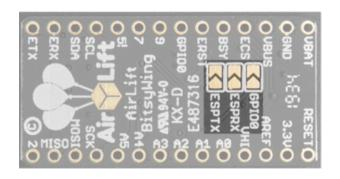
Make sure to solder each of these pads together. You will not be able to upload firmware to your ESP32 if they are not connected.
