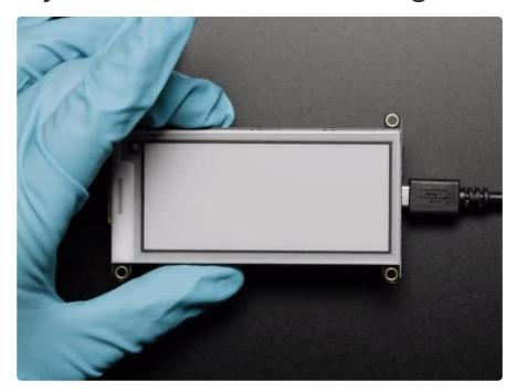
Easy e-paper comes to your Feather with this breakout that's designed to make it a breeze to add a monochrome elnk display. Chances are you've seen one of those new-fangled 'e-readers' like the Kindle or Nook. They have gigantic electronic paper 'static' displays - that means the image stays on the display even when power is completely disconnected. The image is also high contrast and very daylight readable. It really does look just like printed paper!
