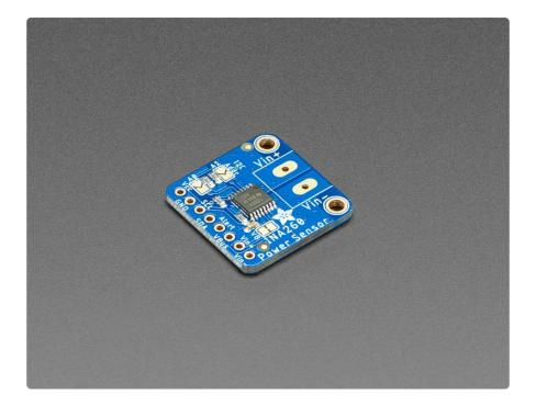
This breakout board may well be the last current sensing solution you every need to buy. Not only can it do the work of two multimeters, but it can do it with amazing precision and flexibility. With it you can measure high or low side DC current, the bus voltage, and have it automatically calculate the power. It can do so over impressive voltage, current, and temperature ranges with better than 1% accuracy, all while delivering the data in an easy to use format over I2C.
