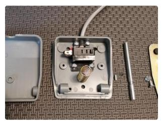
Slowly release the pressure between the two halves of the pedal. When you open it up, be sure to save the spring that provides the pedal its action.
