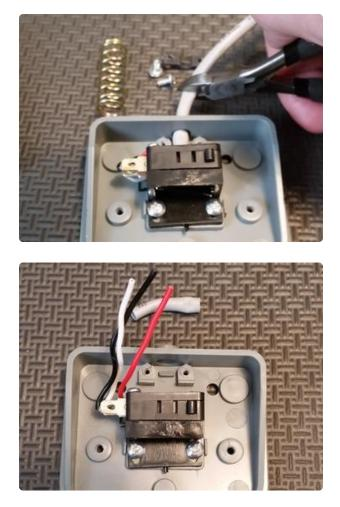
Using wire cutters, cut the cable about 1.5 inches (4 centimeters) past the pedal base.
