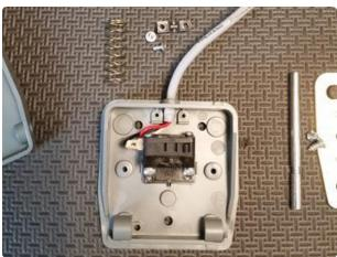
Note the cable restraint - black with 2 screws, holding the cable onto the pedal base in the above picture. Using your screwdriver, carefully remove the two screws and the black plastic bracket holding the wire. Do not remove the switch assembly in the center of the base yet.
