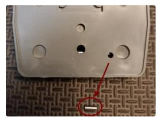
Carefully tip the pedal over and catch the small metal pin. Place it in a safe place with the screws.
