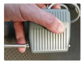
Hold the pedal together with one hand while putting your screwdriver on the metal hinge pin. Keep pressure on the pedal (it is spring loaded) while using pressure to push the hinge pin out.
