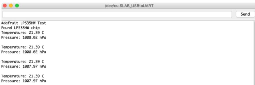
Temperature is calculated in degrees C, you can convert this to F by using the classic  $F = C * 9/5 + 32$  equation.
