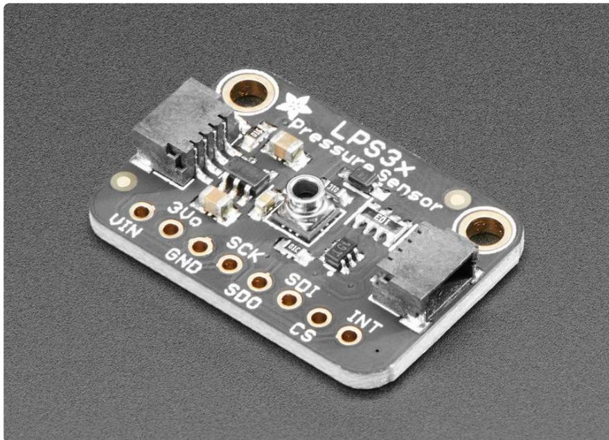
The LPS35HW has a fraternal twin, the LPS33HW. In nearly all respects the LPS33HW is the same as the LPS35HW however the LPS33HW has a bonus feature: a nozzle that can be used to seal it against an enclosure or perhaps a properly fitted tube of some sort. You'll want to make sure to use an appropriately sized o-ring to ensure a good seal. Like the LPS35HW, the LPS33HW chip inside is encased in a protective gel, however in the case of the LPS33HW, the gel is mentioned as being
