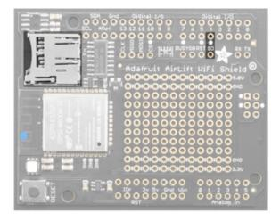
There's a lot of space available on this shield so we also stuck on a micro SD card holder, great for datalogging or storing data to transmit over WiFi.
