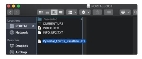
The lights should flash again, BOOT will disappear. Your board should re-enumerate USB and appear as a COM or Serial port on your computer. Make a note of the serial port by checking the Device Manager (Windows) or typing <code>ls/dev/cu\*</code> or <code>/dev/ty\*</code> (Mac or Linux) in a terminal.
