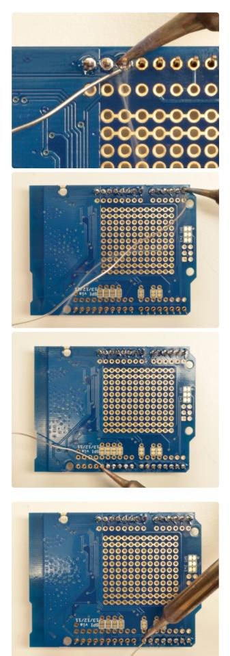
Once you've tacked and straightened all the headers, go back and solder the remaining pins for each header.
