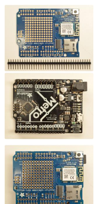
Break apart the 0.1" header into 6, 8 and/ or 10-pin long pieces and slip the long ends into the headers of your Arduino.
