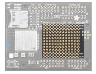
We have a big grid of prototyping holes and power rails if you want to make some custom circuitry!
