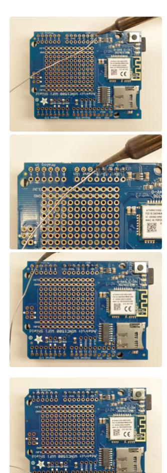
Solder each one of the pins into the shield to make a secure connection
