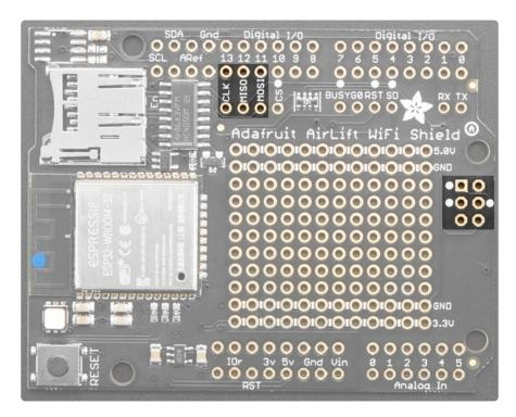
Both ESP32 and SD card use SPI to send and receive data. These pins are labeled CL K MISO MOSI and have level shifting so you can use this shield with 3.3V or 5V microcontroller boards.
