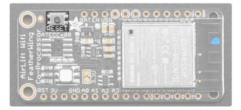
Tap this button twice to enter the bootloader. If it doesn't work on the first try, don't be discouraged. The rhythm of the taps needs to be correct and sometimes it takes a few tries.
