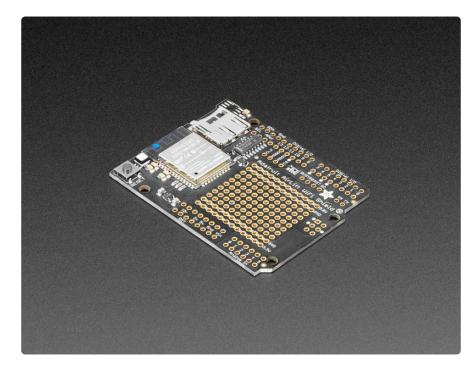
We placed an ESP32 module on a shield with a separate 3.3V regulator, and a tri-state chip for MOSI so you can share the SPI bus with other shields. We also tossed on a micro SD card socket, you can use that to host or store data you get from the Internet. Arduinos based on the ATmega328 (like the UNO) cannot use both the WiFi module and SD library at the same time, they don't have enough RAM. Again, we recommend an M0 or M4 chipset for use with Arduino, M4 for CircuitPython!
