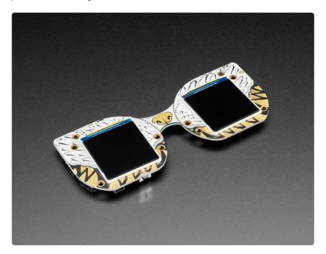
There's also plenty of sensors built in - light sensor, 3 tactile buttons, and a capacitive touch pad on the nose.
