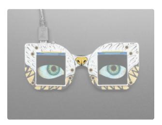
Front and center, is a capacitive touch pad nose this is connected to D2. It's not a great capacitive touch input, because of the zener diode on D2's protection circuitry, but it can detect presses with some startup-calibration. Use as an input.
