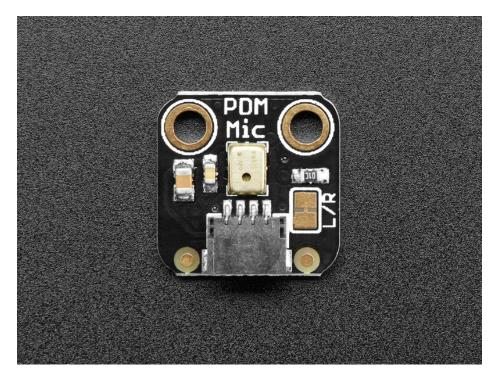
The 4-pin JST connector has **3V**, **GND**, **DAT**, **CLK** connections that can be used with one of our JST-SH cables to make a flexible mic arrangement (https://adafru.it/FGS). If you want a version with breakout headers, we have a version here (https://adafru.it/FBO). An on-board solder jumper lets you change the mic from Left to Right channel
