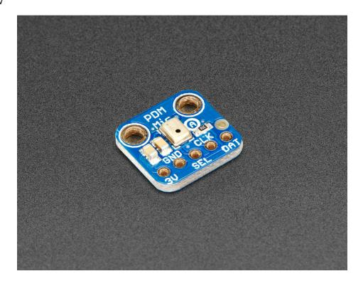
An exotic new microphone has arrived in the Adafruit shop, a **PDM MEMS Microphone!** PDM is the 'third' kind of microphone you can integrate with electronics, apart from analog or I2S. These microphones are very commonly used in products, but are rarely seen in maker projects. Still, they have some benefits so we thought we'd offer a breakout for the shop.
