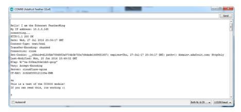
If you don't get an IP address, check you have a green link light, and that your Ethernet is going out to an internet connected router. You may also have to set up the MAC address to allow it access, check with your system admin if you're not sure.
