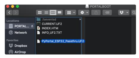
The lights should flash again, **BOOT** will disappear. Your board should re-enumerate USB and appear as a COM or Serial port on your computer. Make a note of the serial port by checking the Device Manager (Windows) or typing **ls /dev/cu\*** or **/dev/ty\*** (Mac or Linux) in a terminal.
