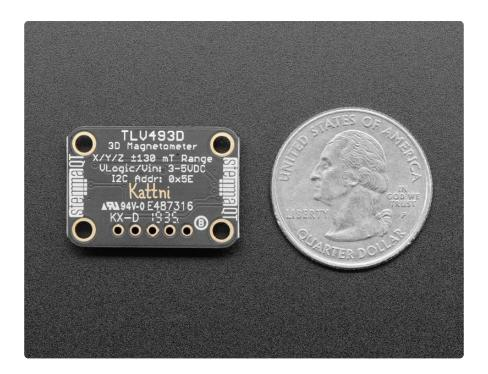
As we are wont to do, we've made the TLV easy to use by putting it on a breakout PCB along with the circuitry to support it. A voltage regulator and logic level shifting combine to make it usable with a range of microcontrollers with either 3.3V or 5V logic levels. We even give you a pin for you to use the excess 3.3V juice not needed by the TLV493D.
