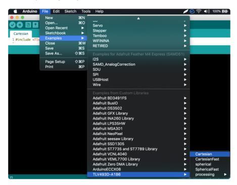
Once you compile and upload the example to your Arduino compatible board of choice, open the serial monitor, verify that your baud rate setting matches the example, and you should see measurements for the three axes being printed. If you wave a magnet near the sensor you can see the values changing!
