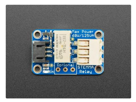
No worrying about flyback diodes, level shifting, pin protection. The STEMMA board takes care of all that for you. You can use it with any 3V or 5V microcontroller/
