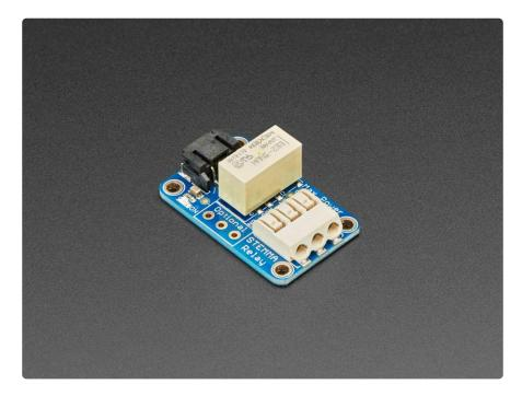
Each STEMMA board comes with a fully assembled and tested PCB but no cable. No soldering is required to use it. There's an optional second switch on the side of the PCB, <u>if you get a 3-pin terminal block</u> (https://adafru.it/GA3) you can solder that in place, but its optional.
