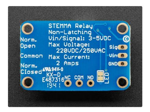
This board has a single Signal pin (the white wire). Normally, the relay's COM pin is connected mechanically to the NC pin and the NO pin is disconnected.
