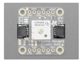
On both sides in the middle are the Sparkfun Qwiic (https://adafru.it/ Fpw) compatible STEMMA QT (https://adafru.it/Ft4) JST SH connectors, for using with I2C. Use with any of the STEMMA QT cables available in the Adafruit shop to connect this breakout to your project without needing to solder!
