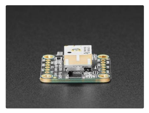
Best of all, we added all the extra goodies you could ever want: a ultra-low dropout 3.3V regulator so you can power it with 3.3-5VDC in, 5V level safe inputs on UART and I2C, a footprint for optional CR1220 coin cell to keep the RTC running and allow warm starts, a green power LED and a tiny red PPS LED. The LED blinks at about 1Hz when a fix is found and is off when no fix.
