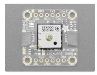
The PA1010D GPS module with built-in antenna is located in the center of the board. It has all kinds of features!
