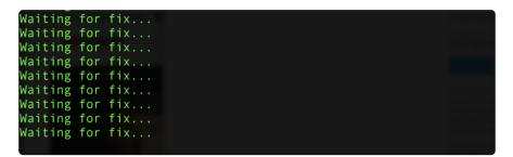
Note: Due to the antenna being built in, the PA1010D Mini GPS module may need a more unobstructed view of the sky than other GPS modules with eternal antennae. With any GPS module, if you are having trouble getting a fix, try moving it to a more ideal location.
