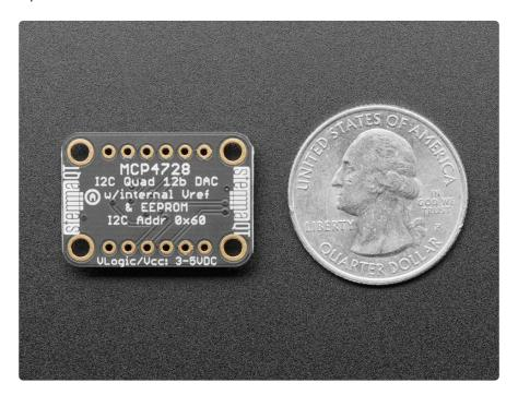
To take things even further, the MCP4728 lets you chose between two sources for your reference voltage: the input voltage that you use to power it on the VCC pin, or an internal 2.048V reference voltage. If you use the internal reference voltage (Vref in
