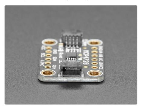
The breakout for the MCP4728 is populated with the required support circuitry to use it with your microcontroller of choice or Blinka-supported computer. The <a href="SparkFun">SparkFun</a> <a href="Qwiic">Qwiic</a> (https://adafru.it/Fpw) compatible <a href="STEMMA QT">STEMMA QT</a> (https://adafru.it/Ft4) JST SH connectors ease the process of connecting the MCP4728 to your project and allows you to easily share an I2C bus with other STEMMA QT, Qwiic, Grove or other compatible sensors.
