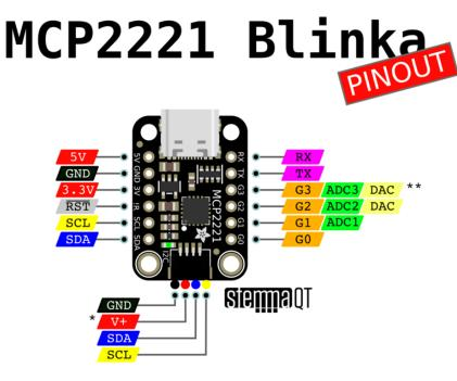
\* 3.3V or 5V as set by jumper \*\* same DAC output on both pins
