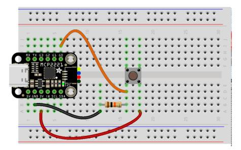
The GPIO pins do not have internal pull-up or pull-down support! If you need pull resistors, add them externally as shown here!
