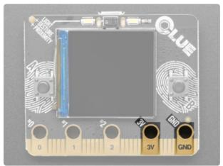
3V and GND - These are the power and ground pads used when connecting external sensors etc. typically using alligator clips.
