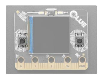
• A and B buttons - The CLUE has two user-programmable buttons on the front, labeled A and B. Use them as inputs to control your code. These are unconnected when not pressed, and connected to GND when pressed, so they read LOW. Set the pins to use an internal pull-UP when reading these pins so they will read HIGH when not pressed. Buttons can be addressed in CircuitPython using board.BUTTON A and board.BUTTON B, and in Arduino as D5 (left button) and D11 (right
