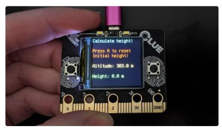
The Adafruit CLUE has a barometric pressure sensor that uses the pressure readings to calculate altitude. For more information on how this works, check out <u>Wikipedia</u> (ht tps://adafru.it/J2e).
