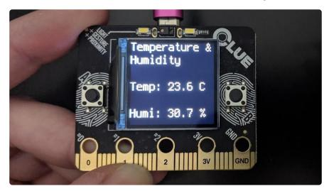
The Adafruit CLUE has a temperature and humidity sensor that reads the temperature in degrees Celsius and the relative humidity in percent. To learn more about relative humidity, check Wikipedia (https://adafru.it/CxM).
