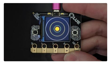
The Adafruit CLUE comes with a built in accelerometer for measuring acceleration. For more information on how that works, check out Wikipedia (https://adafru.it/J2d).
