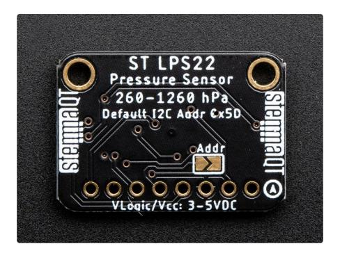
Furthermore, we've included <u>SparkFun Qwiic</u> (https://adafru.it/Fpw) compatible <u>STEM MA QT</u> (https://adafru.it/Ft4) connectors for the I2C bus so you don't even need to solder! All you need to do is plug in a <u>compatible cable</u> (https://adafru.it/JnB), wire it up to your device using one of our wiring diagrams and you're ready to write some code to start reporting measurements.
