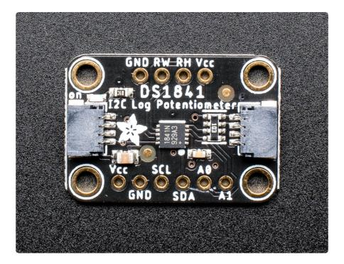
Potentiometers are the perfect tool when you want to change your circuit by turning a knob. Turns out, there are times when you want to adjust your circuit without manually turning a knob, and the DS1841 I2C Logarithmic Resistor from Maxim can do just that. It's a programmable resistor, similar to an I2C potentiometer like the the DS3502 I2C Potentiometer (https://adafru.it/HDc), so why another?
