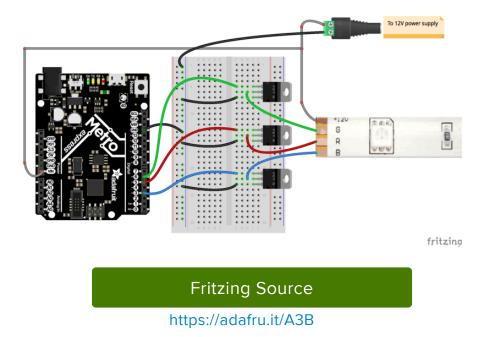
Note: Be sure to use PWM output pins from your board! Not all digital inputs/outputs support PWM output. Check your board's guide and pinout to confirm. Typically a PWM-capable output will have a dot or wavy signal line next to it on the board's silkscreen.
