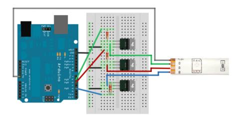
Connect a 9-12V power supply to the Arduino so that Vin supplies the high voltage to the LED strip. If you want, you can also just use a separate wire that connects to a power supply that provides about +12V. Make sure to connect the ground of that
