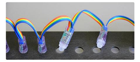
LED pixels can be press-fit into holes drilled through metal, wood or plastic. Holes 11 to 12 millimeters in diameter seem about right — experiment on a piece of scrap material first, find a size that gives a firm but not damaging grip.
