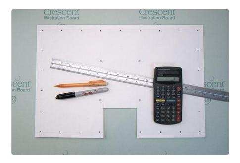
Next, calculate the spacing for a ring of 25 LEDs. For this monitor, it worked out nicely as a 9x6 rectangle, roughly 2" spacing, with a one pixel gap at the bottom where the monitor stand protrudes. Perfect!
