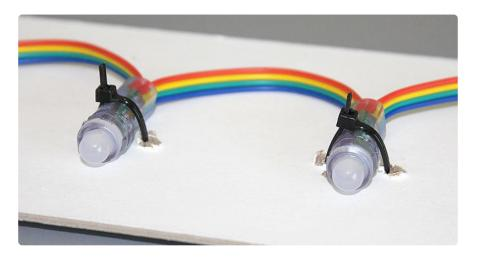
Cable ties work well with pixels on their side. Holes can be made using an awl, or you can make very clean holes using a leatherworking punch.
