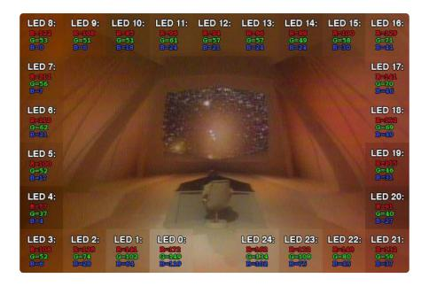
If you plan to arrange the LEDs similarly to our examples — 25 pixels in a ring, 1 pixel gap at the bottom, with the first pixel starting just left of the gap — then nothing more needs to be changed in the software. If using a different layout, you'll need to make adjustments in the code. You'll find extensive notes in the source code for making this (and other) changes.
