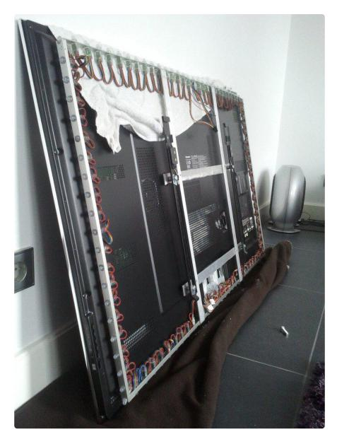
Forum user "Wackid" made this stunning 100 LED Adalight frame using aluminum Utrack with drilled holes carefully spaced around the perimeter. Extreeeeme!
