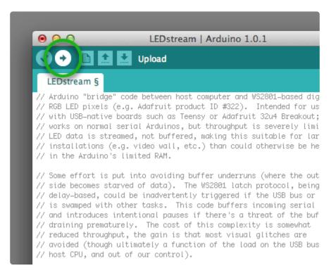
After the code is uploaded, if the LEDs are correctly wired up and the power supply is plugged in, the LEDs should all flash red, green, then blue for about a second each, then off. This is a startup diagnostic that tells you the LEDs and Arduino are working
