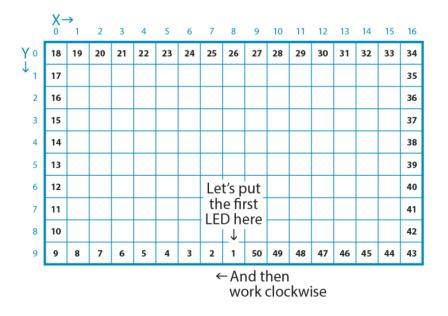
(This is the view from the front of the screen. When installing the LEDs on the back, you'll want to mirror the layout, flipping everything left-to-right.)
