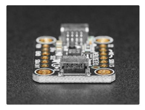
The breakout for the LIS331 family takes one of these little dynamos and puts it on a custom made PCB in the <a href="STEMMA QT">STEMMA QT</a> form factor (https://adafru.it/LBQ), making them easy to interface with. The <a href="STEMMA QT">STEMMA QT</a> connectors (https://adafru.it/JqB) on either side are compatible with the <a href="SparkFun Qwiic">SparkFun Qwiic</a> (https://adafru.it/Fpw) I2C connectors. This allows you to make solderless connections between your development board
