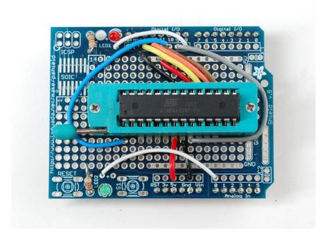
Finally, you'll need to solder on the header to allow the shield to be placed on, break the 0.1" male header and place it into the Arduino sockets. Then place the shield above on top to solder it in place.
