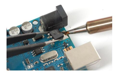
Clean up the tabs and remove any clipped parts still stuck on.
