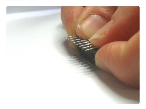
Finally, replace the old chip, lining up all the pins and making sure that the notch in the chip matches the notch in the socket!
