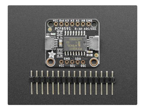
Along with four 8-bit ADC channels, the PCF8591 comes complete with an 8-bit Digit al to Analog Converter converter as well! Not only can you measure voltages, but now you can create them just as you want them. You can even use the DAC and ADC together to create an input to a circuit and measure the results with the ADC. The possibilities abound!
