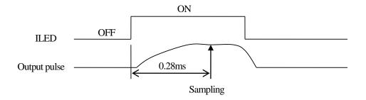
3-4 Recommended input condition for LED input terminal
