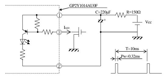
(\*4) Sampling timing of output pulse
