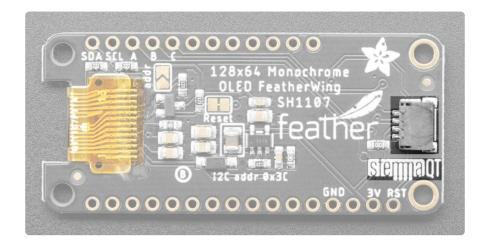
We've even included a <u>SparkFun qwiic</u> (https://adafru.it/Fpw)-compatible <u>STEMMA QT</u> (https://adafru.it/Ft4) connector for the I2C bus so you can plug and play any of our STEMMA QT, qwiic or <u>Grove I2C</u> (https://adafru.it/Ndk) sensors and devices! Check out the available sensors and devices on the Adafruit shop (https://adafru.it/HMF).
