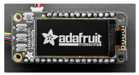
It's easy to use the Adafruit 128x64 OLED FeatherWing with CircuitPython and the Adafruit CircuitPython DisplayIO SH1107 (https://adafru.it/OaL) module. This module allows you to easily write CircuitPython code to control the display.
