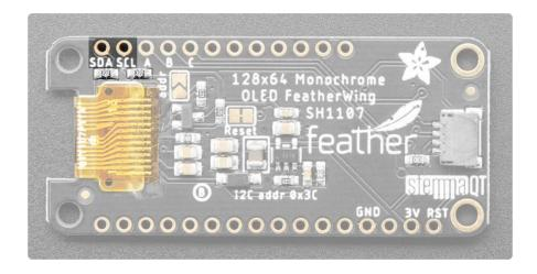
The cute little OLED does all of the data transfer over the I2C pins, highlighed above SDA and SCL. No other pins are required. There are two 2.2K pullups to 3V on each.
