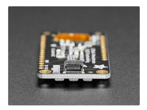
Tested working with all Feather boards. The OLED uses only the two I2C pins on the Feather, and you can pretty much stack it with any other FeatherWing, even ones that use I2C since that is a shared bus.
