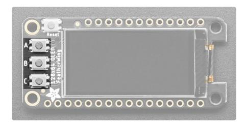
The button pins ON THE BACK are labeled incorrectly in the initial revision of this FeatherWing. It should read C, B, A from left to right, where C should be next to SCL.
