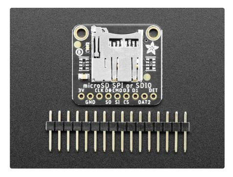
With the Adafruit MicroSD SPI or SDIO Card Breakout Board, you can add an SD card to your project using the common SPI interface or the higher performance SDIO interface.
