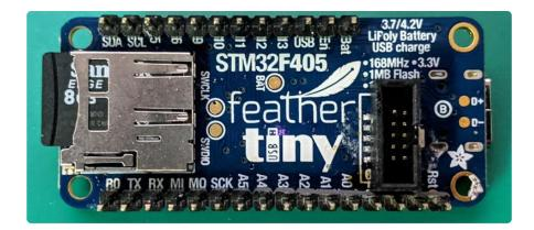
The Feather STM32F405 Express uses SDIO to connect its built in micro SD card slot. Didn't notice it had an SD card slot? We hid it on the underside.
