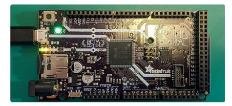
The Adafruit Grand Central M4 Express has a built-in SD card connected to the SPI bus, so no wiring or soldering is needed!
