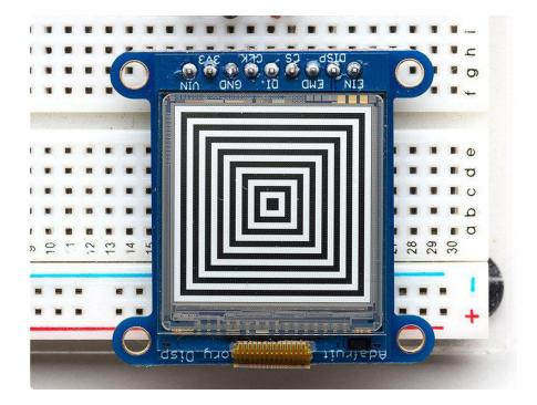
The 1.3" SHARP Memory LCD display is a cross between an elnk (e-paper) display and an LCD. It has the ultra-low power usage of elnk and the fast-refresh rates of an LCD. This model has a matt silver background, and pixels show up as little mirrors for a silver-reflective display, a really beautiful and unique look. It does not have a backlight, but it is daylight readable. For dark/night reading you may need to illuminate the LCD area with external LEDs.
