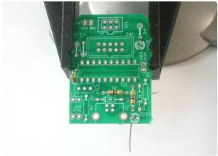
Next up are the 2 47 ohm resistors. Place them as shown. Bend the legs out, flip the PCB, solder the 4 joints and clip them.
