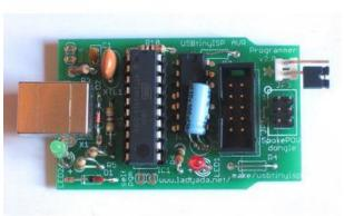
Now that you have a lot of practice with resistors, you can do the remaining 5 all at once. Place R10 (10K pullup resistor), R3, R5 and R6 (1.5K resistors for the USB connection, LEDs and output buffer).
