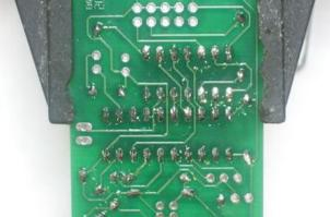
Next to be placed is the 74AHC125 buffer. This chip does a level-shifting conversion on signals from the USBtiny microcontroller to the device being programmed. This way you can safely program chips that vary from 1.8V to 5.5V voltage.
