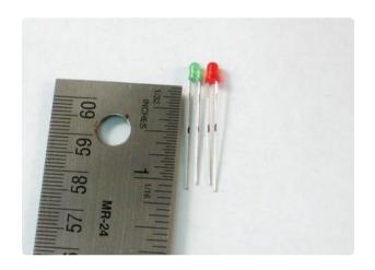
The two LEDs are next. They should stand-off a bit from the PCB so make a marking about 1/2" (1cm) from where the colored plastic ends.
