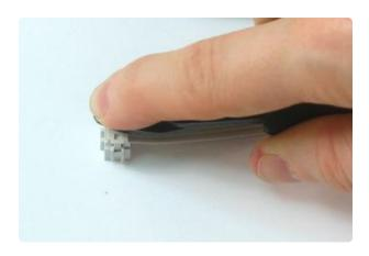
Do not use needlenose pliers to try to press the pieces together. You have to have very flat pressure from both sides.
