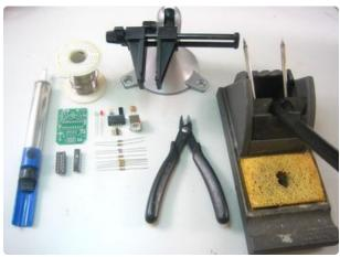
Get your tools ready! A board vise, soldering iron & solder, diagonal cutters, and a solder sucker (desoldering tool) if you have one.
