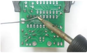
Tack two opposite corners of the socket, to keep it in place, and then solder all the pins.
