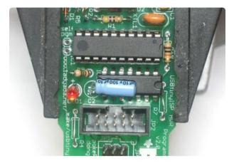
Finally, straighten the pins of the microcontroller and place it, so that the notch in the chip matches the notch in the socket (and the silkscreen) as shown.
