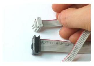
It's important that the key (the bump in the connector) and the red stripe line up. Match the image on the left, just poke the conductor in with a mm or two past the edge.
