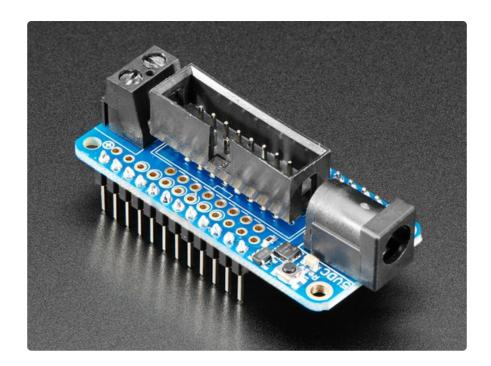
This wing can be assembled in one of two ways. You can either solder in a 2x8 IDC shrouded header on the top, then plug in the IDC cable that came with your matrix. This makes it easy to stack on top of your Feather. Or, you can solder in the 2x10 socket header on the bottom of the Wing, and then stack your Feather on top. That way you can plug it directly into the back of the matrix \*mind blown\*
