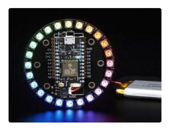
There's also a 24-pixel RGB ring (http://adafru.it/2268) specifically designed for the Particle (formerly Spark) Photon development board.
