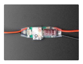
A buck converter (https://adafru.it/efD) can efficiently step a higher DC voltage down to 5V for NeoPixels and microcontrollers ... for example if you have a 12V power source, like a car battery.
