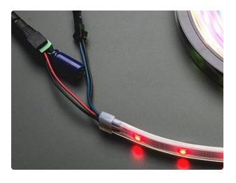
Before connecting a NeoPixel strip to ANY source of power, a large capacitor ( $500-1000~\mu F$  at 6.3~Volts or higher) across the + and – terminals provides a small power reservoir for abrupt changes in brightness that the power source might not otherwise handle — a common source of NeoPixel "glitching."
