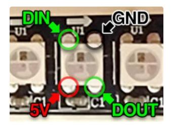
Some batches of 144 pixel strip don't have pads between the LEDs. If you cut these into shorter sections, the only way to connect to them (except at the halfmeter segments) is to carefully solder directly to the LED. The corner with the notch is the GND pin.
