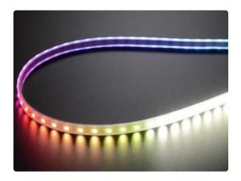
A recent addition is RGBW NeoPixel strips. These add a fourth LED element — pure white — which is more "true" and pleasing to the eye than white mixed from red+green+blue. Like the RGB strips, they're available in different pixel densities and backing strip colors.
