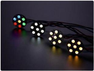
All measure 23 millimeters (0.9 inches) in diameter.
