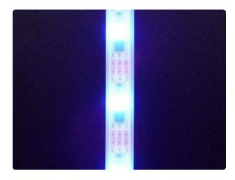
A single-color ultraviolet variant of NeoPixel strip is available for special applications, currently one pixel density and backing color:
