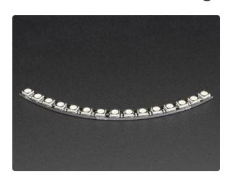
Though originally designed to be used in groups of four to complete a 60 NeoPixel Ring, the individual 15-pixel quarter rings can also be used to solve interesting design problems! RGB and RGBW are available.
