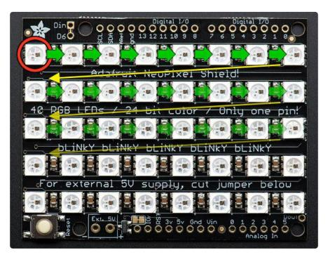
We refer to this layout as row major and progressive. Row major means the pixels are arranged in horizontal lines (the opposite, in vertical lines, is column major). Progressi ve means each row proceeds in the same direction. Some matrices will reverse direction on each row, as it can be easier to wire that way. We call that a zigzag layout.
