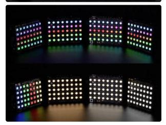
This 5x8 NeoPixel Shield for Arduino (http://adafru.it/1430) fits neatly atop an Arduino Uno or compatible boards (5V logic recommended). Like many of our NeoPixel products, they're available in RGB and various RGBW pixel types:
