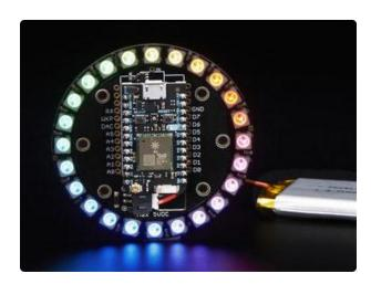
Previously mentioned on the "Rings" page, but for posterity: this 24-pixel RGB ring (http://adafru.it/2268) is specifically designed for the Particle (formerly Spark) Photon development board.
