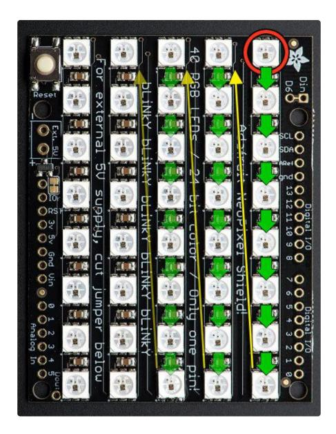
Now the first pixel is at the top right. Pixels increment top-to-bottom — it's now colum n major. The order of the columns is still progressive though.
