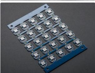
These are similar to the sewable Flora NeoPixels, but with a pin arrangement that (with the addition of headers) fits neatly into a breadboard for prototyping. Also available in two formats:
