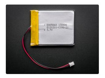
For many wearable projects we recommend a lithium-polymer battery (http://adafru.it/328). These deliver 3.7 Volts — perfect for directly feeding low-power microcontrollers such as the Adafruit Flora, yet enough voltage to run a short length of NeoPixels.
