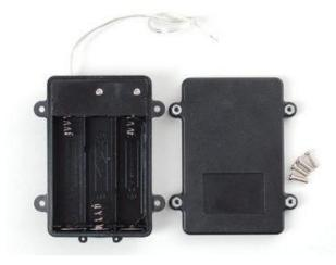
Three alkaline cells (such as AA batteries) can be installed in a battery holder (http://adafru.it/771) to provide 4.5 Volts. Though larger and heaver than the fancy lithium-polymer pack, they're inexpensive and readily available.
