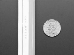
This distinctive NeoPixel flex strip has a gorgeous diffused neon-like appearance thanks to its thick silicone casing.
