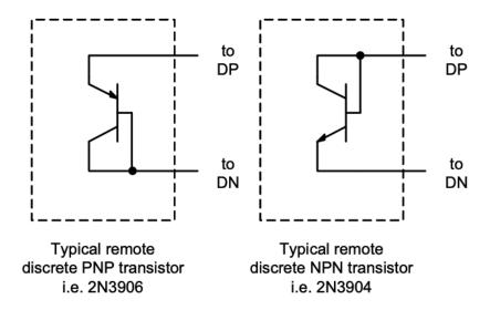
I've put diode in quotes above because we've only been able to successfully measure external temperature using a NPN BJT transistor with the collector and base tied together which acts like a diode. PNP BJT's should also work with the base and emitter connected. The diagram from the datasheet above shows how connecting the pins of a BJT lets it act like a diode.
