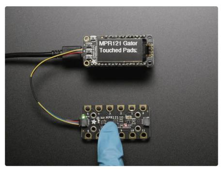
Add lots of touch sensors to your next microcontroller project with this easy-to-use 12channel capacitive touch sensor breakout board, starring the MPR121. This chip can handle up to 12 individual touchpads with plug-and-play STEMMA QT connector and large alligator/croc-clip friendly pads, it's a no-solder solution to capacitive touch sensing.
