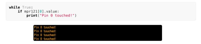
If you don't see any messages when you touch the inputs, you might need to ground yourself to the board by touching the GND pin on the board with one finger and then touching the input pads with another finger.
