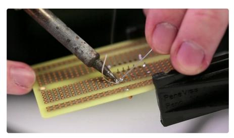
Because perfboard gives us access to the bottom side of our circuit, we can use the long component leads themselves to make some of the connections which required jumpers before.
