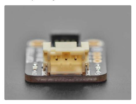
Note that this board is specifically for proximity sensing or break-beam projects. While it can receive 38KHz IR remote control signals - there isn't a filter system so you'll get a lot of spurious signals.
