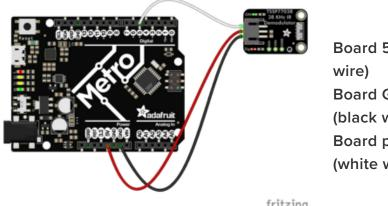
Board 5V to demodulator JST PH V+ (red Board GND to demodulator JST PH GND (black wire) Board pin 5 to demodulator JST PH Sig (white wire)
