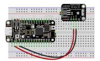
Board 3V to demodulator VIN (red wire) Board GND to demodulator GND (black wire)
