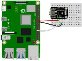
Pi 3V to demodulator VIN (red wire) Pi GND to demodulator GND (black wire) Pi GPI05 to demodulator SIG (white wire)
