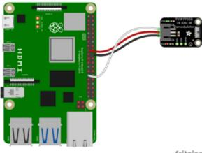
Pi 3V to demodulator JST PH V+ (red wire) Pi GND to demodulator JST PH GND (black wire) Pi GPIO5 to demodulator JST PH Sig (white wire)
