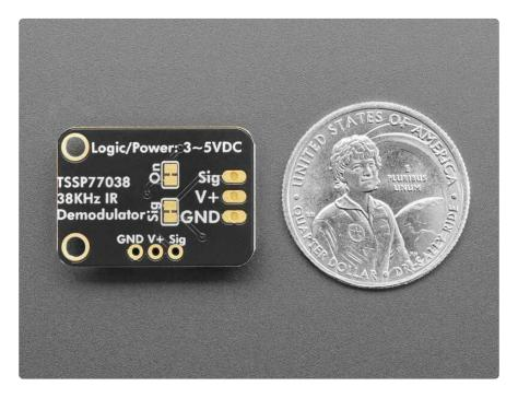
This board will work nicely for a variety of IR detecting projects, and with mounting holes and a cable, a lot easier to mount in enclosures and on devices. Using a 2mm pitch STEMMA JST PH cable with headers or alligator clips on the end, you can easily wire this board without any soldering.
