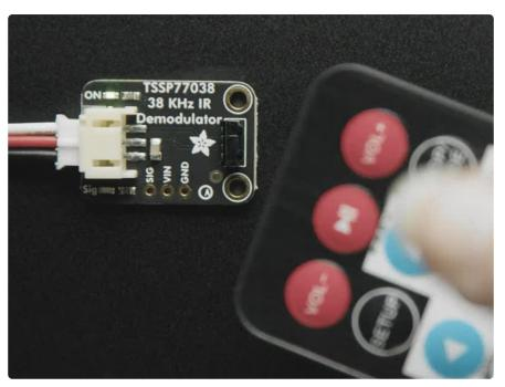
While designing our <u>IR decoding breakout</u> (http://adafru.it/5939), we noticed the <u>TSSP</u> series of chips from Vishay (https://adafru.it/19UA). These are simpler than more 'remote control' receivers in that they don't do any filtering on the codes received: you really just get the demodulated-from-38KHz-signal output.
