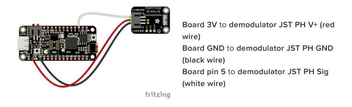
The following is the demodulator wired to a Feather RP2040 using a solderless breadboard:
