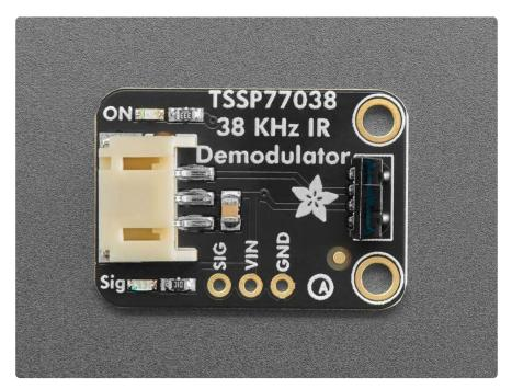
According to Vishay, they're designed for "Reflective Sensing, Light Barriers, and Fast Proximity Applications". These sensors could be interesting for use when you want a less-'intelligent' IR decoder, or for proximity projects where you don't want to go all-out for a VCNL I2C sensor (http://adafru.it/4161).
