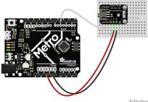
Board 5V to demodulator VIN (red wire) Board GND to demodulator GND (black wire)
