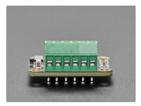
Then **A-** and **A+** pads connect to the differential outputs from the bridge. For example, connecting to a strain gauge these tend to be the white and green wires. If you have a second gauge or voltage you want to measure, you can use the **B-** and **B+** pads. On the A channel, you can select 64x or 128x gain. On the B channel, you have a fixed 32x gain.
