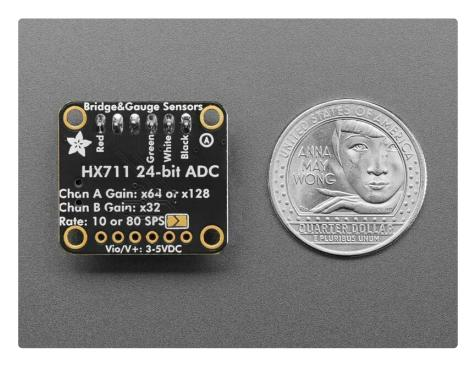
Each breakout comes with a HX711 ADC chip, plus some support circuitry, and 6 port terminal block that can be used to connect one or two 4-wire sensors. The **E**- pad
