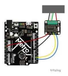
Strain gauge power to breakout E+ (red wire)
