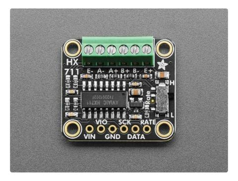
If you are feeling the stress and strain of a Wheatstone bridge and you want to quantify it, this handy breakout will do the job, no sweat! The **Adafruit HX711 Breakout** contains a super-high-resolution 24-Bit differential ADC with extra gain circuitry that makes it perfect for measuring strain gauges / load cells or other sensors that have four wires that are connected in a Wheatstone bridge arrangement (https://adafru.it/-kd).
