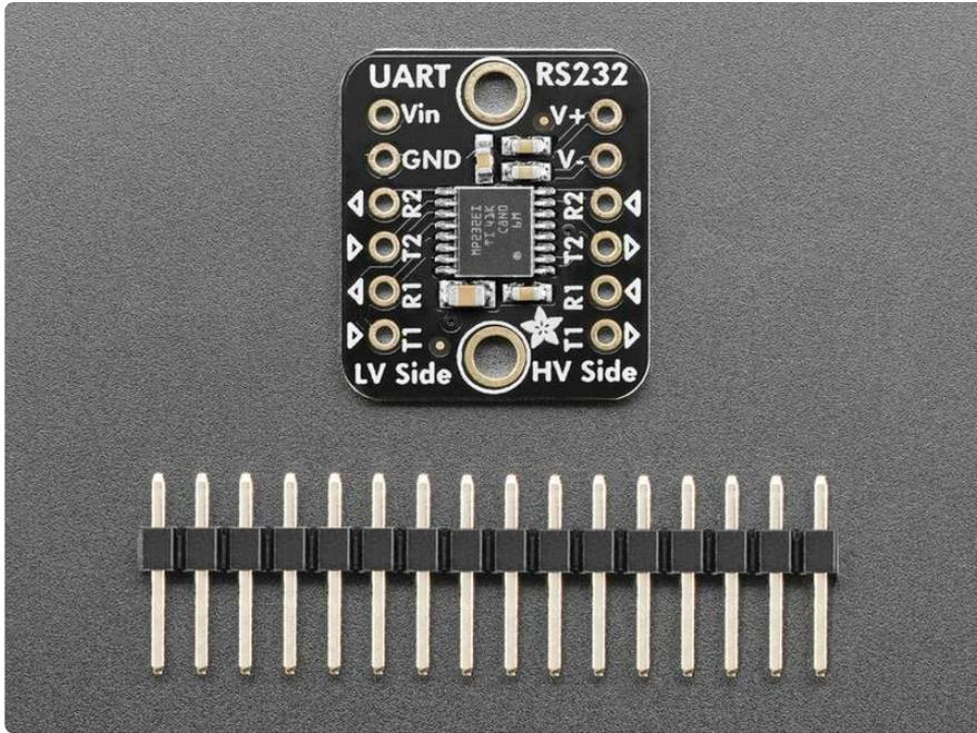
If you want to use a microcontroller or microcomputer to chat with a RS-232 then thankfully all you need is a serial port / UART (something just about any microcontroller has) and a level shifter. The level shifter is required because while most UARTs are 0-3.3V or 0-5V logic level, RS-232 requires +6 to +10V, yep the signal voltage goes negative! That means a specialized shifter is required, one that can generate the extra high and low voltages and also safely convert the logic levels.
