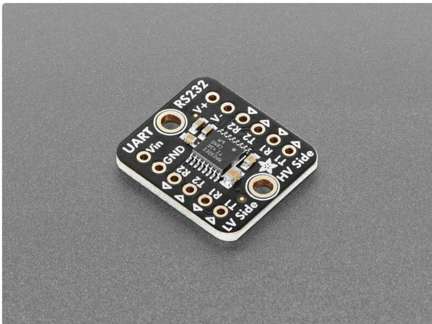
Sure you could buy a raw [MAX232 chip \(https://adafru.it/1a46\)](https://adafru.it/1a46) and wire up the necessary capacitors, but this board does it all for you plus it can run on 3.3V power and logic, which many older chips can't do. It also can do 2 duplex channels, so you can have both RX and TX plus two flow control pins like RTS and CTS.
