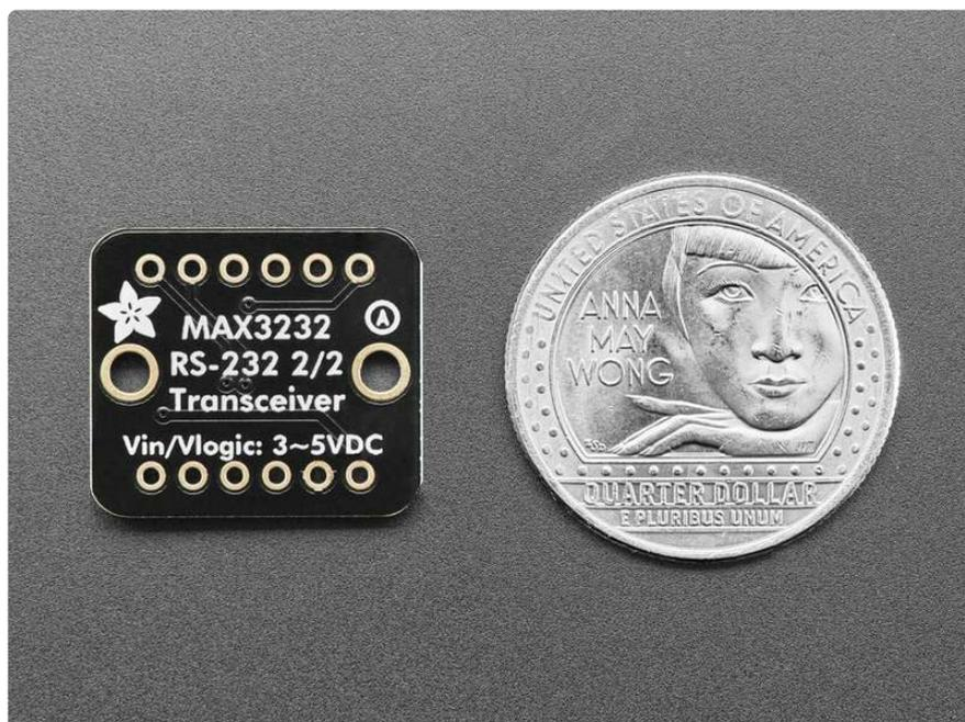
RS-232 is what we had before USB: a 9 or 25 pin D-Sub connector that would allow data plus flow control lines. Many folks may remember these interfaces were used for mice, modems, barcode scanners, tele-types and more. We still find devices sold that have RS-232 ports, although [many folks use a USB to RS-232 adapter \(https://adafruit.it/1a45\)](https://adafruit.it/1a45) these days.
