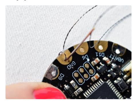
Bring your needle from front to back through the hole in the circuit board. Pull the needle and slack thread all the way through until the thread snugly hugs the conductive pad ad the edge of the board.
