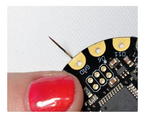
Bring the needle through the fabric from back to front, right next to the circuit board.
