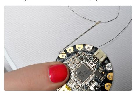
Pull the needle all the way through and continue pulling the thread tail until only 6 inches remains at the back of the fabric.
