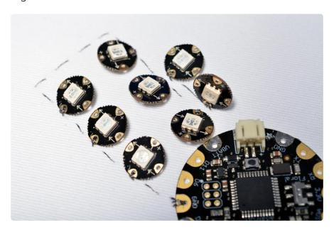
Now that all the pixels are anchored by one pad, clean up any stray threads on the back.
