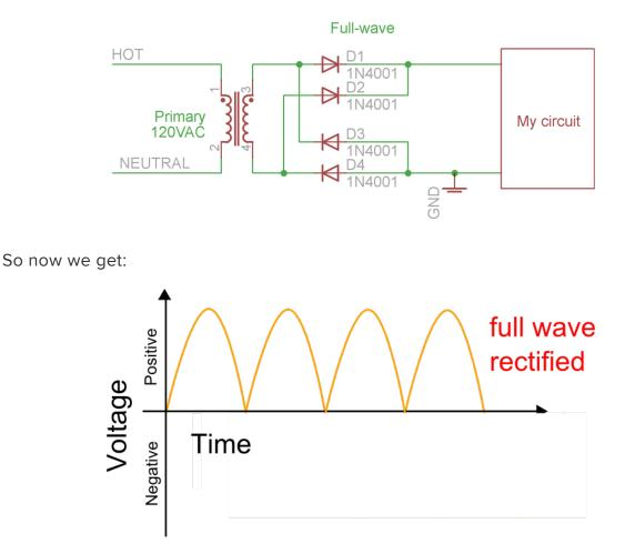
As you can see, there are twice as many humps - there isnt that "half the time, no voltage" thing going on. This means we can divide the calculated capacitor size to half of what it was in the previous.
