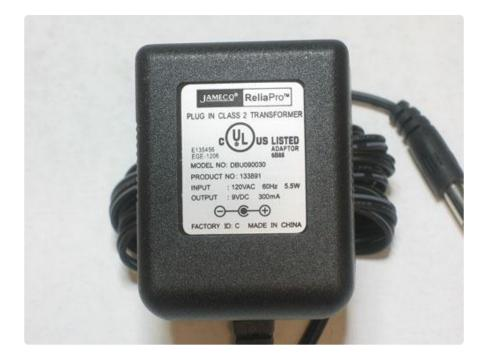
These guys are everywhere - all sorts of voltage and current ratings. They're available for sale at any store just about, but there are some big things to watch out for! One is that the output voltage is not going to be 9V (for example) out of the box, that voltage rating is just the minimum output for the current rating (200mA for example). And also, the output is going to have a lot of ripple on it!
