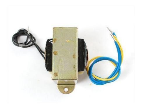
We aren't going to get into the heavy detail of the electromagnetic theory behind transformers except to say that they are made of two coils of wire around a chunk of iron. If the number of coils are the same on both sides then the AC voltage is the same on both sides. If one side has twice the coils, it has twice the voltage. They can be used 'backwards' or 'forwards'! For more detailed information, be sure to check out the wikipedia page (https://adafru.it/alf).
