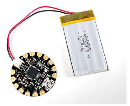
More advanced users may wish to use a rechargeable <u>lithium polymer battery</u> (http:// adafru.it/258) for their smaller size and longer duration. These batteries pose added risk if abused, shorted, bent, crushed, or punctured. FLORA does not have onboard charging, so you would also need a separate LiPoly charger (http://adafru.it/259).
