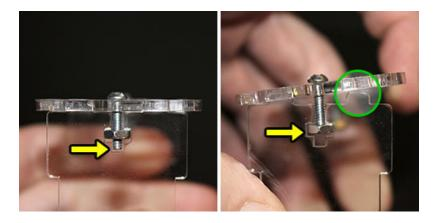
Insert the BeagleBone base plate into the case by inserting the alignment studs into the back face, then pivot the
