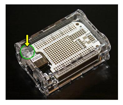
Press the front face flush again and tighten all the screws. Acrylic is brittle, so don't crank these down too hard – finger pressure plus 1/8 turn is sufficient. Insert the microSD card (make sure it goes into the card slot, NOT loose in the case!). Bingo...you're done!
