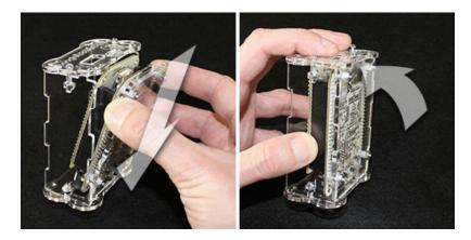
Now tip the face plate in the opposite direction and install the case top in a similar fashion. Align the hole in the top face with the reset button on the BeagleBone (once sealed, this is accessed with a paper clip or small screwdriver). Or you can choose to keep the top cover off, if you'll need frequent access to the BeagleBone or cape.
