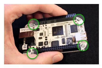
Flip the board over, using fingers and thumb to hold the screws in place. If this is a dexterity challenge, the screws can also be held with tape:
