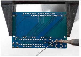
Solder each leg, taking care not to accidentally 'short' two button legs together. The ones for the directional pads are very close!
