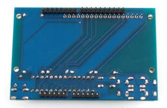
Flip over the shield and place it flat on the table so the long leads of the header stick out.
