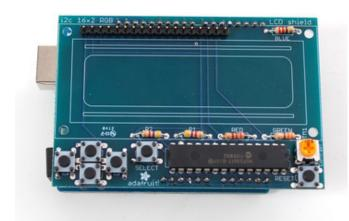
Next, check if you have an RGB LCD (with 18 pins) or a Monochrome display (not RGB, with 16 pins).
