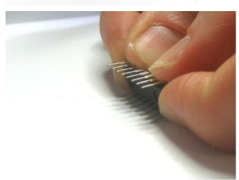
We're nearly done! Now we will place the I2C port expander chip. Double check that it has the MCP23017-E/SP marking on it. This is a 16-pin expander chip, that uses the i2c bus. That means you can send it commands using the i2c pins on an Arduino and control 16 more digital pins! 5 of those pins go to the buttons, 6 go to the LCD control and 3 are used for the backlight (the remaining 2 are unused).
