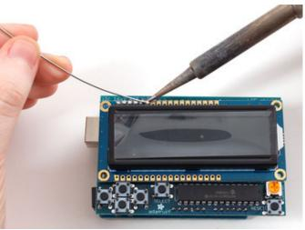
Solder all the pins to the LCD display.
