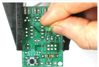
Now it's time to place the small indicator LED **LED5**. LED's are not symmetric and must be placed correctly in order to work. You'll notice one leg of the LED is longer than the other. This is the *positive* leg. The positive leg goes into the hole with a + next to it. In the picture shown, its the left hole.
