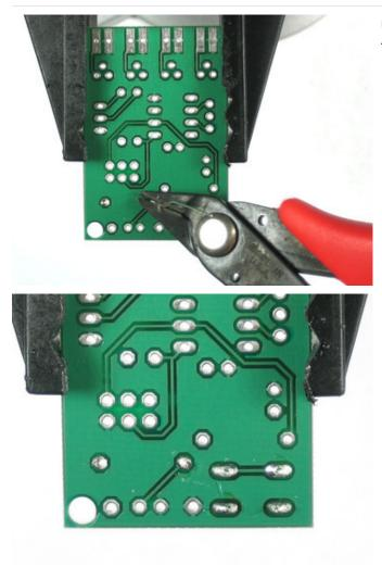
Use the diagonal cutters to clip off the resistor legs so that only the solder points remain.
