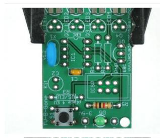
Next, place 2 components. The ceramic oscillator and the 8-pin socket. The oscillator has 3 pins and is symmeteric. The oscillator is the timeclock for the microcontroller, making sure that it is performing its functions at the correct speed.
