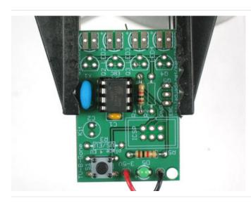
Next place the 1.0K ohm resistors, **R1**. This is the base resistor for the PNP transistor.
