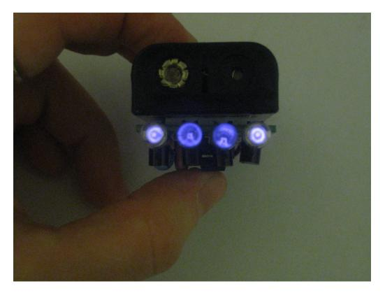
Digital cameras can detect infra-red light but our eyes can't. Use a digital camera, webcam or camcorder and look through the digital viewfinder at the IR LEDs, after pressing the button, the LEDs should flash.
