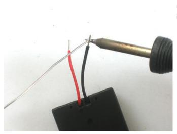
Use your soldering iron to 'tin' the wire, melting solder into it to keep the wire from fraying.
