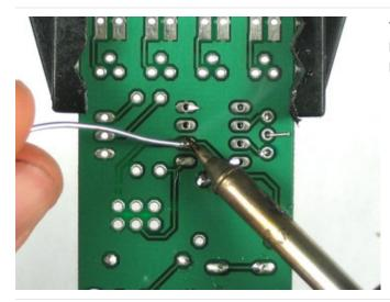
You may need to solder one pin of the socket while holding it it in with a finger (or tape) as the legs aren't long enough to be bent while in place.
