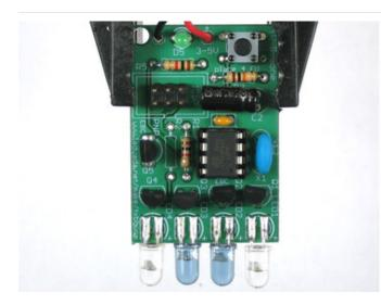
If you're planning to reprogram the chip, solder in the 6pin ICSP header. The long pins go up.
