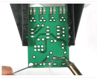
Using your soldering iron, heat up a leg of the button and the poke solder into it to make a nice solder joint.
