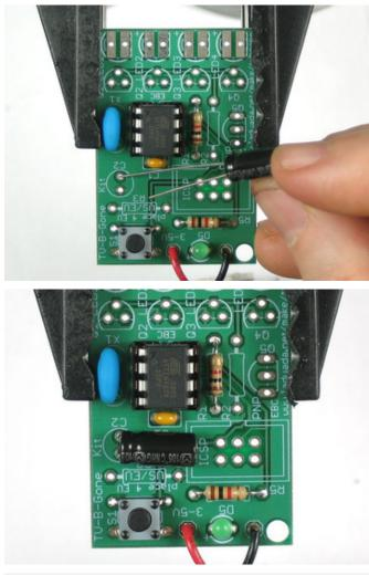
Next is the 220uF electrolytic capacitor. It is polarized so make sure it goes in the right way. The long lead is positive, and goes into the hole marked with a +, on the right in this photo.
