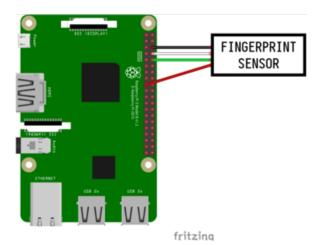
Here's an example using the Pi's built-in UART:
