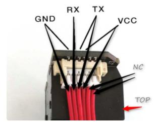
If your sensor is an older one and has all the same-color wires, The first wire from the left is ground, then the two data pins, then power. You'll have to cut, strip and solder the wires.
