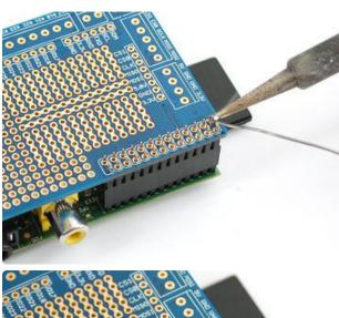
Heat up the soldering iron to 650 °F and wait for it to get up to temperature. Then heat a corner pad/pin with the iron tip and after two seconds poke in a small amount of solder. After the solder has melted into the pad/pin remove the iron.
