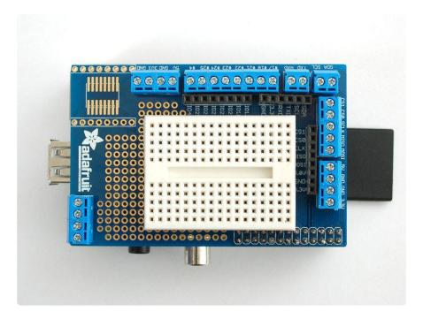
We designed the plates so you can fit a <u>'tiny breadboard'</u> (http://adafru.it/65) on top and still see the pin labels on the breakouts. This makes it easy to do fast prototyping!
