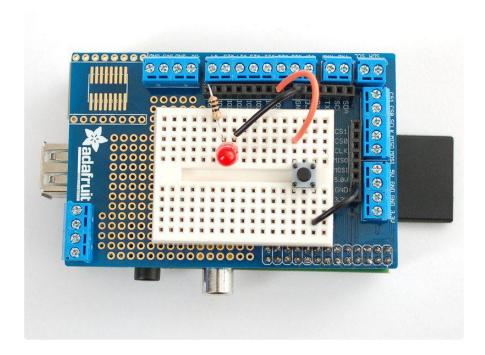
For more permanent projects, you can just place parts in and solder directly into the proto plate
