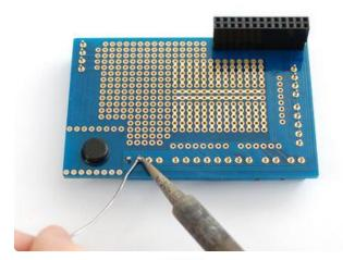
Solder each terminal block connection to the PCB using plenty of solder to make a strong mechanical connection
