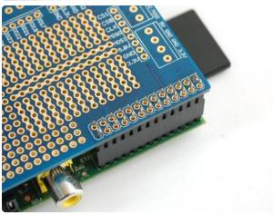
Start by soldering the two corner pins. This will allow you to make sure the plate is aligned properly and fix it if its crooked.
