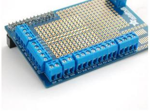
Carefully flip over the PCB, you may need to tape down the terminal blocks with scotch tape if they seem to fall out. With all the terminal blocks in place, it should sit flat on a table.
