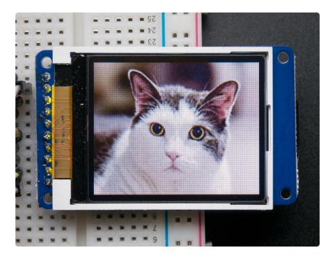
This tutorial is for our 1.8" diagonal TFT display. It comes packaged as a breakout or as an Arduino shield. Both styles have a microSD interface for storing files and images. These are both great ways to add a small, colorful and bright display to any project. Since the display uses 4-wire SPI to communicate and has its own pixel-addressable frame buffer, it requires little memory and only a few pins. This makes it ideal for use with small microcontrollers.
