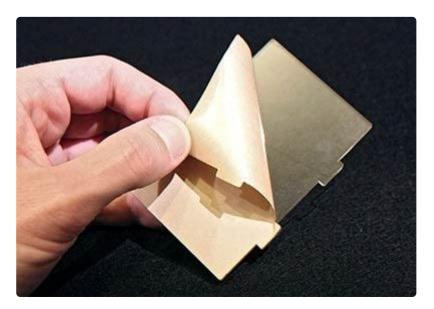
With the paper removed, you'll notice the four sides of the case have I/O ports labeled. This will help later to tell inside from out. Note especially the side with the HDMI port...if you find the case isn't assembling right, it's most often because this side is installed upside-down or inside-out.
