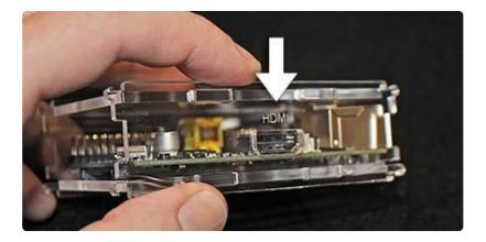
10. Install the first end of the case: slide the top of the end piece over the two top hooks first, then, using very light pressure, pivot the end piece downward over the bottom two hooks. It should click into place without difficulty. If you encounter ANY resistance, stop! Do not force this piece or you will break the plastic. Back off, check the alignment of the other pieces (especially the HDMI side), and try again. Gently. And remember, top to bottom — the other direction will break.
