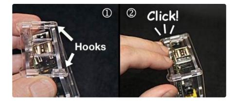
11. Install the opposite end of the case using the same technique. Top to bottom.
